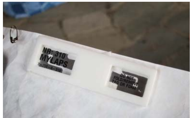
Reverse side of bib number with RF circuit
