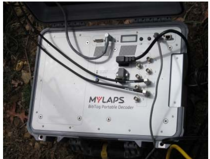
As each runner crossed the finish line and over a pair of antennas, their bib circuit sent a signal that recorded their bib number and finish time
