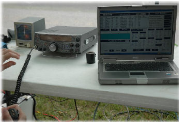
The main operating position with Kenwood TS-2000 transceiver and laptop with FD logging software
