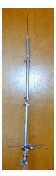
The task at hand now is to match the resonant resistance to a 50 or 75 ohm feed line. For this the PUFF computer aided design program works quite well. It should be obvious that the lower the radiation resistance is, the wider the bandwidth of the antenna will be. Additional elements can be added with appropriate phase reversal to increase gain. The 70 cm antenna has 3 elements and should show about 6 db or better.
