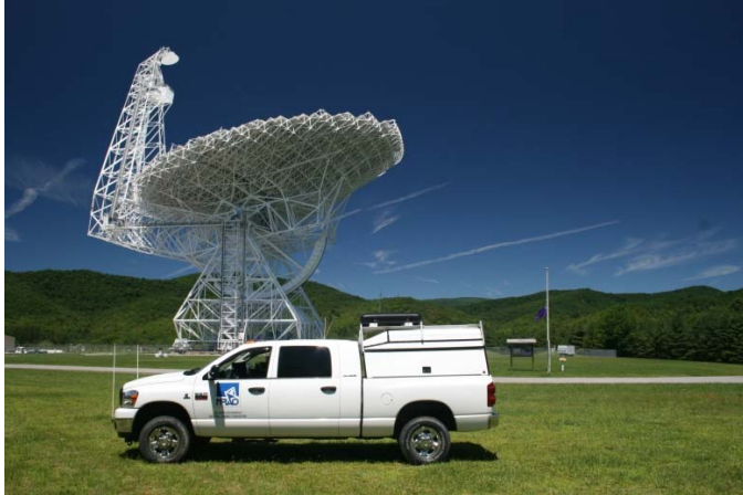
Wes's truck E.M.I.T.T. – ElectroMagnetic Interference Tracking Truck. In the background is the new Robt. C. Byrd GBT- over two acres of surface, 17 million pounds; one of the largest moving structures on earth. Photo by W. Sizemore
