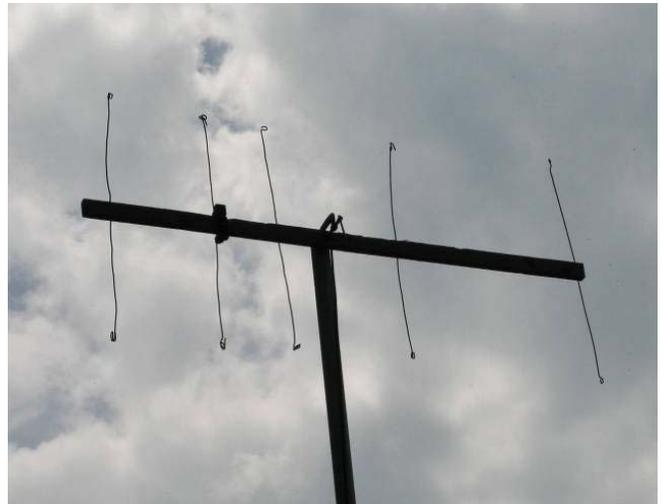
True to science, I started with a dipole driven element, cutting it too long to allow for "tweaking". Then came the reflector. Next the first director which was a bit more trouble to get the SWR down to an acceptable number, requiring tweaking of both the driven element and the
