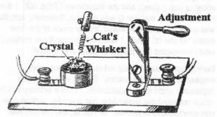
I wired up a detector using a piece of wood to mount all components. I used wood screws with reasonably wide heads. This gave me a way to mount components and secure them. Again, I knew I would need an audio amplifier
